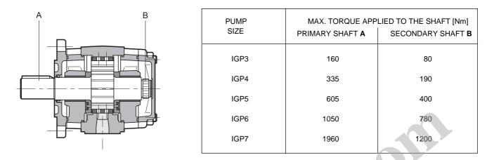
NOTE: The pumps must be connected in order of decreasing displacement and size.
