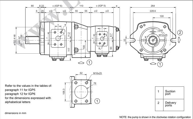
For the anticlockwise configuration, the delivery ports, 2), are on the opposite side of the pump
